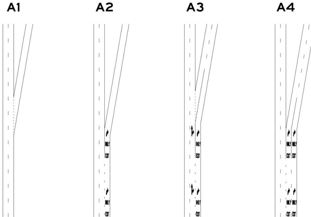
**FIGURE 6** Configurations of Exiting Lanes
