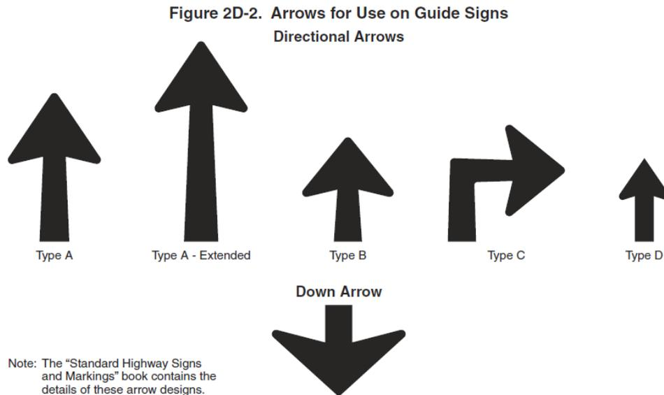
**FIGURE 3** Arrows for Use on Guide Signs, *MUTCD* Figure 2D-2
