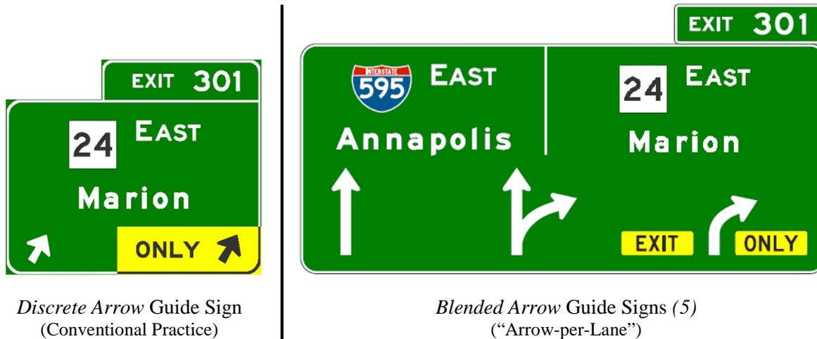
8 **FIGURE 2** Examples of Guide Signs for Option Lane Signing
